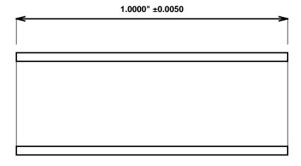
Sintered Bronze Impregnated with Synthetic Performance Difference  $^{\text{TM}}$  AM1-SPD  $^{\text{TM}}$ .
