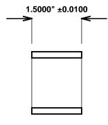
Design Requirement: Boundary Lubrication Application, High Load-Low Speed Applications. Extreme Pressure Lubrication with Moly Additive.
