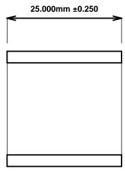
Iron-Based Sintered Product Impregnated with Extreme Pressure Synthetic AM3-SPD™. Higher Load, Slower Speed Designs Economic Alternative Material. Metric
