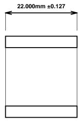
Sintered Bronze Impregnated with Food Grade Mineral Oil: FDA 21 CFR172.878. For Food Contact Applications. Metric.
