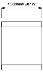
Sintered Bronze Impregnated with Food Grade Mineral Oil: FDA 21 CFR172.878. For Food Contact Applications. Metric.
