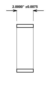
Sintered Bronze Impregnated with Synthetic Performance Difference  $^{\text{TM}}$  AM1-SPD  $^{\text{TM}}$ .
