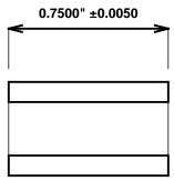
Sintered Bronze Impregnated with Food Grade Mineral Oil: FDA 21 CFR172.878. For Food Contact Applications.
