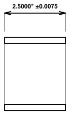
Sintered Bronze Impregnated with Synthetic Performance Difference  $^{\text{TM}}$  AM1-SPD  $^{\text{TM}}$ .
