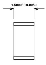
Sintered Bronze Impregnated with Synthetic Performance Difference  $^{\text{TM}}$  AM1-SPD  $^{\text{TM}}$ .
