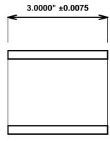
Sintered Bronze Impregnated with Synthetic Performance Difference  $^{\text{TM}}$  AM1-SPD  $^{\text{TM}}$ .
