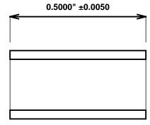
Sintered Bronze Impregnated with Food Grade Mineral Oil: FDA 21 CFR172.878. For Food Contact Applications.
