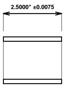
Sintered Bronze Impregnated with Synthetic Performance Difference  $^{\text{TM}}$  AM1-SPD  $^{\text{TM}}$ .
