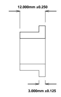
Iron-Based Sintered Product Impregnated with Extreme Pressure Synthetic AM3-SPD™. Higher Load, Slower Speed Designs Economic Alternative Material. Metric
