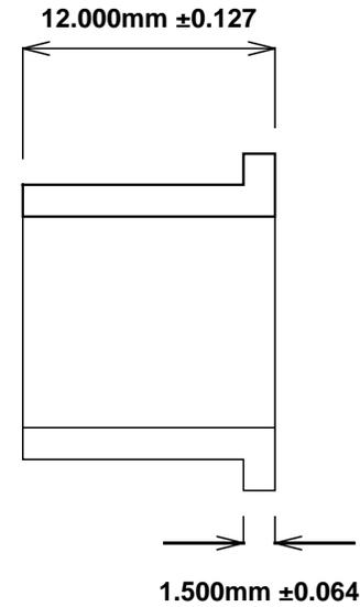
Sintered Bronze Impregnated with Food Grade Mineral Oil: FDA 21 CFR172.878. For Food Contact Applications. Metric.
