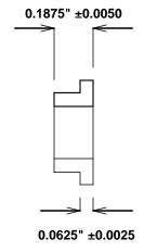
Sintered Bronze Impregnated with Food Grade Mineral Oil: FDA 21 CFR172.878. For Food Contact Applications.
