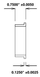
Sintered Bronze Impregnated with Synthetic Performance Difference  $^{\text{TM}}$  AM1-SPD  $^{\text{TM}}$ .
