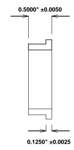
Sintered Bronze Impregnated with Synthetic Performance Difference  $^{\text{TM}}$  AM1-SPD  $^{\text{TM}}$ .
