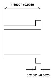
Sintered Bronze Impregnated with Synthetic Performance Difference  $^{\text{TM}}$  AM1-SPD  $^{\text{TM}}$ .
